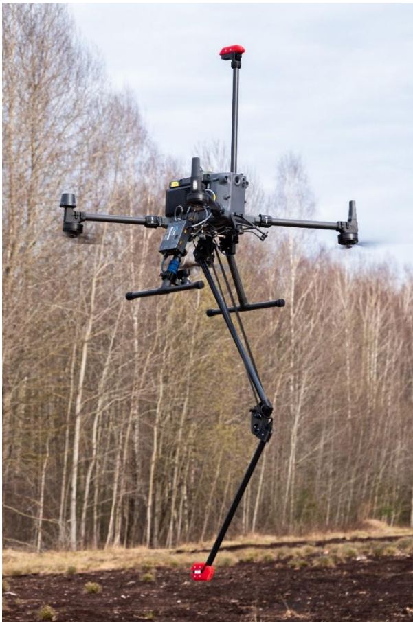
Image: MagNIMBUS in gradiometer configuration in flight
