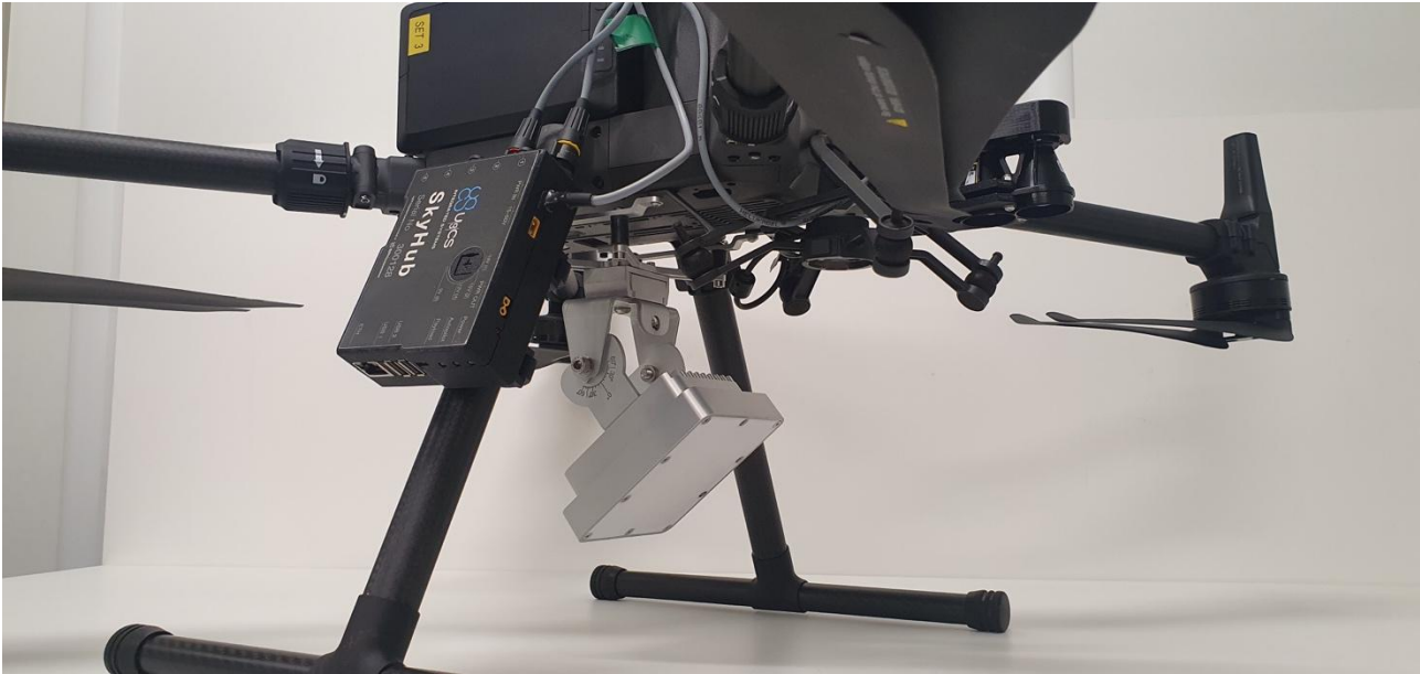
Figure 2: Geolux RSS-2-AB surface velocity radar payload installed on the UAV
